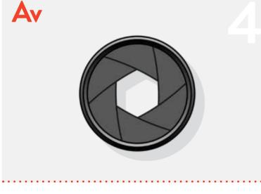
Av mode, or Aperture priority mode, allows the photographer to set a fixed aperture while letting the camera decide the best corresponding shutter speed and ISO to achieve a well-balanced exposure for your output.
