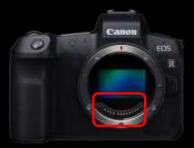
The EOS R system uses 12-pin electronic contacts to provide significantly improved communication between the camera and lens. Information such as the focus, zoom, aperture, and IS is instantly transmitted to the camera.
