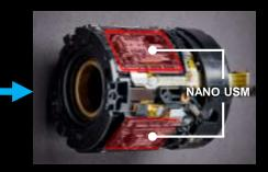
This is the first Canon model to use electronic floating focus control with two NANO USM units. Independent operation of the focusing lens group and floating lens group reduces the minimum focusing distance for improved close-up shooting and further AF precision improvements.
